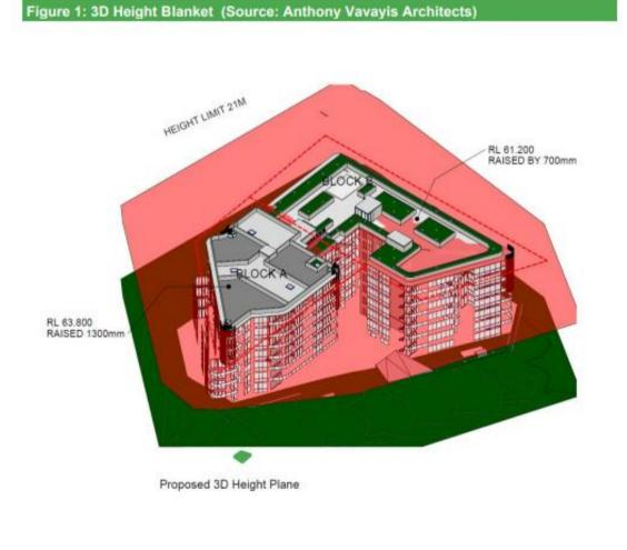
The approved development varied the 21m SEPP height control with an approved height of 23.38m to the highest lift overrun.
